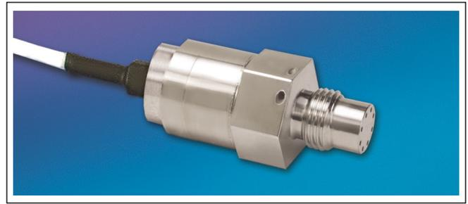
ETL-375 Series transducers are miniature, threaded instruments. The sensing sub-assembly is protected from mechanical damage by a solid screen which has been shown to have minimal influence on the frequency response of the sensor. The ETL Series uses Kulite's Patented Leadless Technology.
