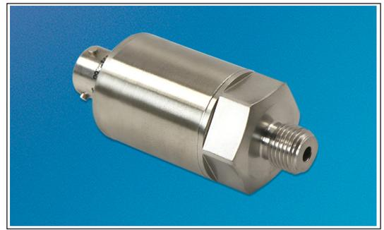
The IPTE-483-1000 offers a high accuracy voltage output with a total error band of 0.25% FSO across the ultra-wide temperature range of -40°C to +150°C. Designed to measure liquid or gas pressure (with its all-welded, hermetic stainless steel construction), the transducer is ideal for road test, flight test and industrial sensing applications.
